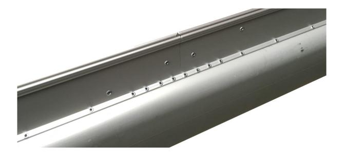
The bottom section of sail track will need cutting to length at the position where the track finishes (mark X). Once cut to the finished length, deburr the track end and radius the sides carefully. Luff tape damage could result if the track end is not deburred and the luff groove is not rounded off.
