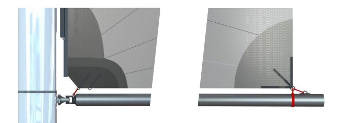
Use the electrical winch or use the winch handle (inserted into the spool face plate) to roll the sail onto the <u>port side</u> of the mandrel (clockwise when facing aft). Two persons should assist by pulling either the luff or leech, so as to ensure the bolt rope remains in the area between the boom edge and the mast, whilst the sail is being furled.
