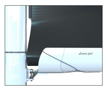
In the instance where the sail works forward, increase the resistance on the main halyard and ensure the sail is unloaded.
