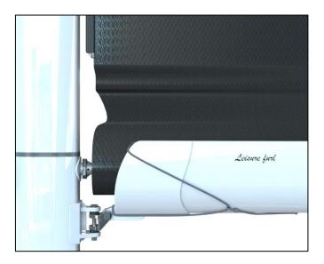
Do not release the main halyard in spurts. The balance of resistance is essential for efficient furling.
