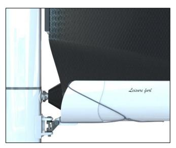
If the sail shows these signs of substantial pull back, reduce the resistance on the main halyard. You will immediately notice that the lines of pull back gradually disappear as you continue.
